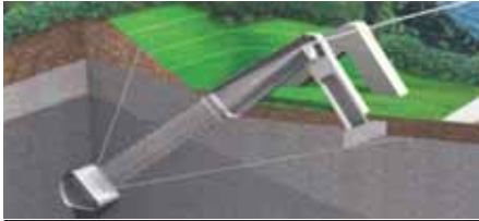
Earth anchorage using the intact rock mass
