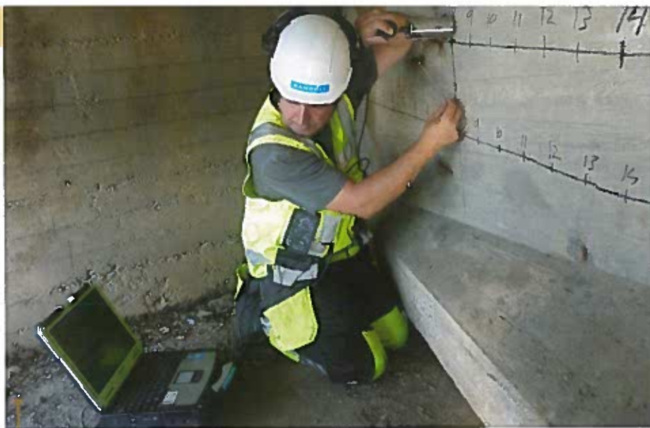
NDT- Impact-Echo testing
